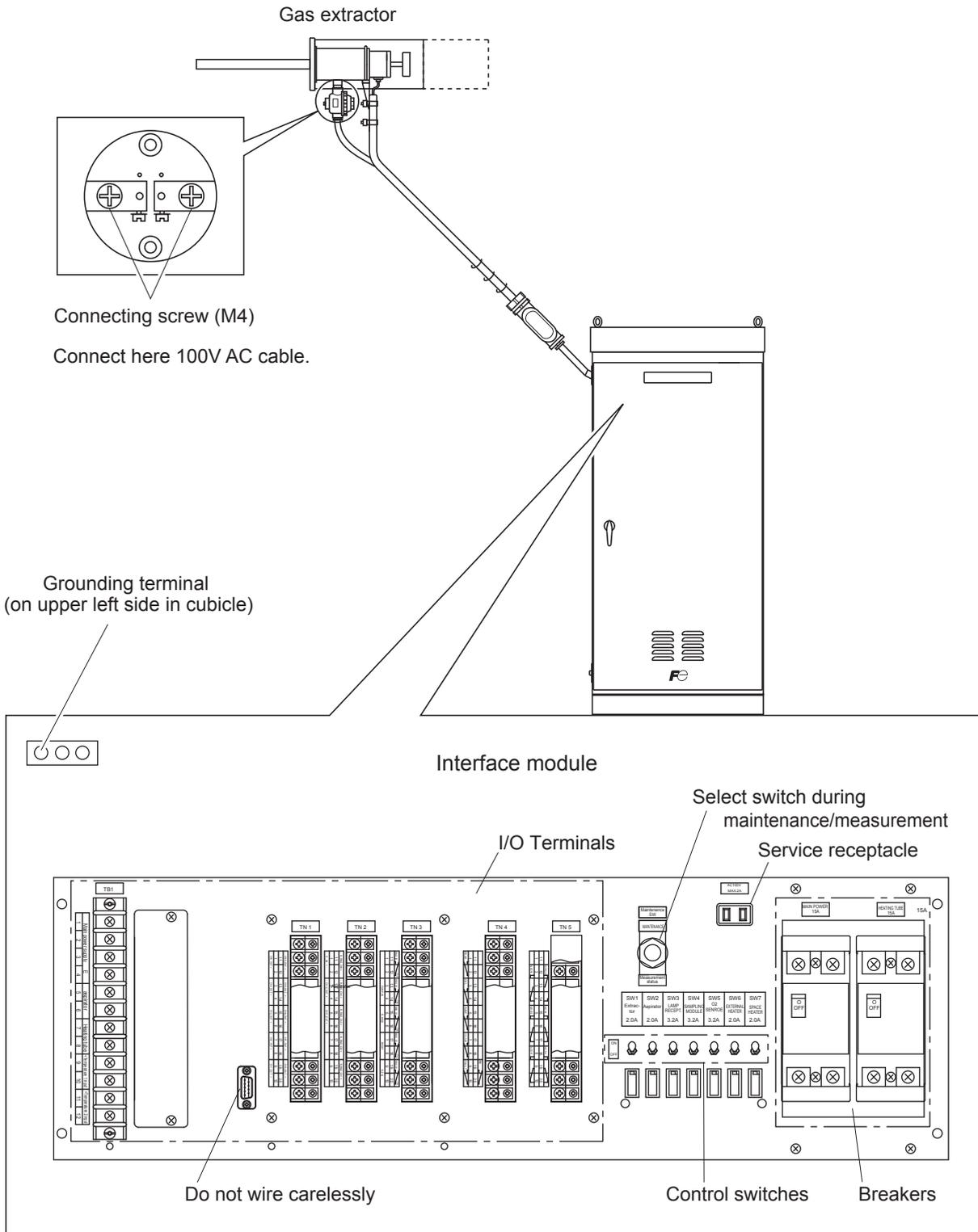
Fig. 3-1 Wiring procedure
