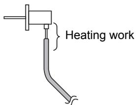
**Note) Use the heating tube in cold climate or if SO<sub>2</sub> analyzer is included.**
