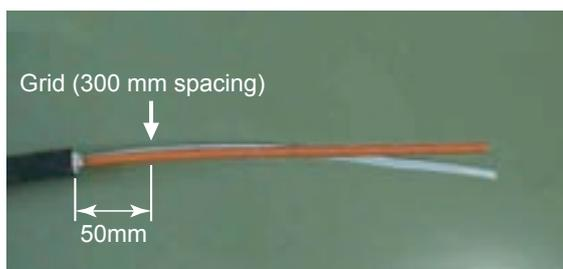
**Note) Paying attention not to damage the process tube nor heater wires, cut the altogether to a certain degree, and pull it out forcibly.**
